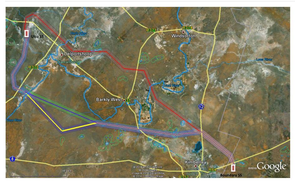
Figure 7: Google Earth image with the proposed alternative routes for the Boundary to Ulco power line and the delineated aquatic features
